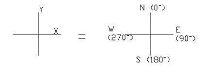
Each shot has a North-South (or Y) component and a East-West (or X) component we must find to put it on the plot. This too is trig
