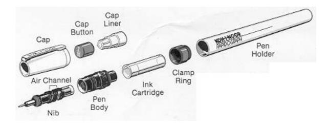
They are fairly easy to use. You fill a reservoir with the correct ink for the job (depending on the material you are drawing on), shake the pen up and down (over a piece of scrap paper) a few times, and off you go! The pens have a reservoir, a weight with a wire attached, and a tip - very little else.
