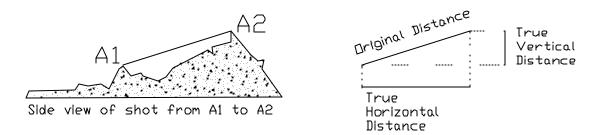
The formulas to generate these distances are Trig and are based on the Inclination (So that's why we take inclination!)
